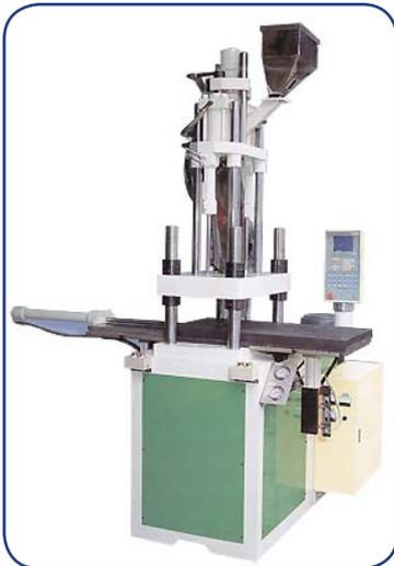
Basically we used Vertical Injection Molding Machine. This machine configuration allows manufacture plastics parts with metal elements inserts. The advantages of vertical injection molding have gained a lot of converts. Production molds for it has considerably simplified design, and for production run of a new product it is required to make only new mold templates and ejector pins that considerably reduces time of new parts manufacturing and the cost price of a final product at all.
